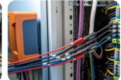
Arrows on all clamps have to be pointed towards the electrical load. • Pay close attention to connecting the analyzer in
